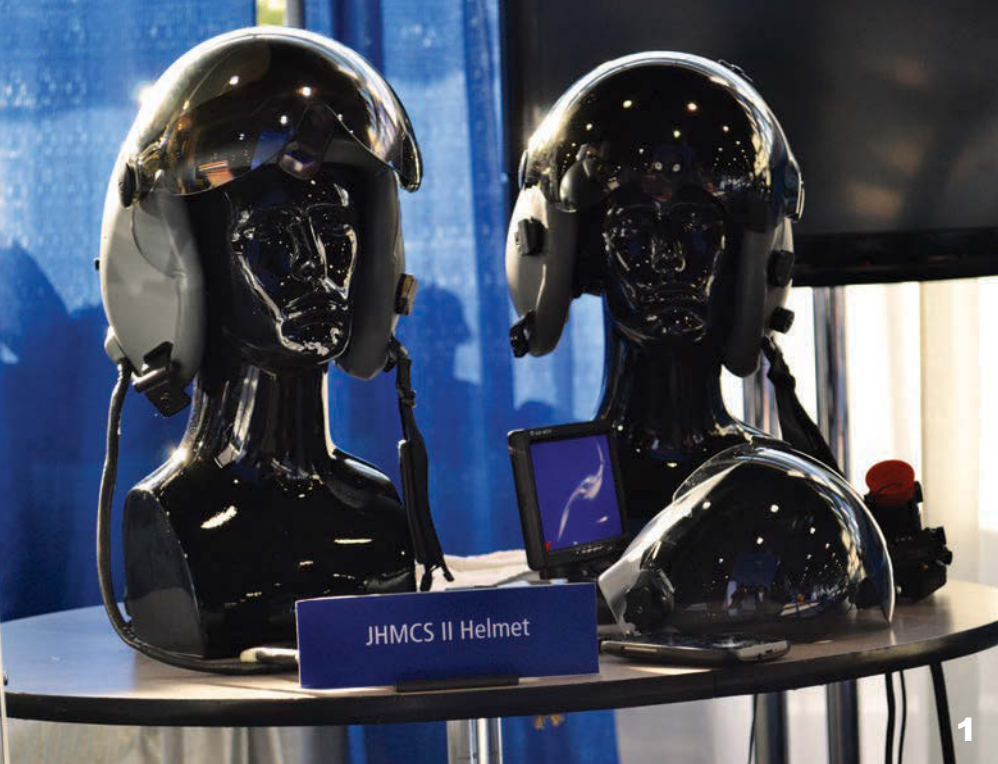
111 Elbit's Joint Helmet-Mounted Cueing System headgear sparkles in the exhibit hall. The helmets are used on Air Force F-16s to give pilots better situational awareness and the ability to select targets merely by looking in their direction. 121 This Wideband Gapfiller satellite model orbited above Boeing's booth. 131 Raytheon displayed an Advanced Combat Radar, one of a number of active electronically scanned array radars for a possible F-16 upgrade. 141 CMSAF James Cody (left) talks with Col. Jaak Tarien of the Estonian air force. Air Chiefs from 18 countries attended the ASC 2014 Tech Expo. Tensions in Europe and the Middle East seemed to spark serious interest among foreign visitors.
